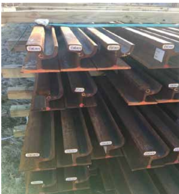
Figure 1: Oklahoma Streetcar Project welding 51R1 rail from Voestalpine
