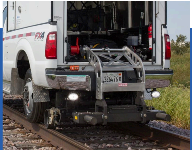
The Argus® track geometry system mounted on 800-series TrackSTAR® vehicle
