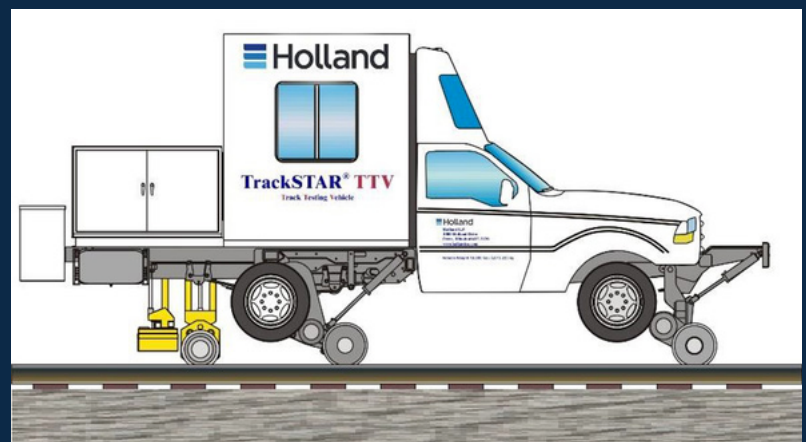
TrackSTAR® 491, Holland's Track Testing Vehicle (TTV), designed for transit systems
